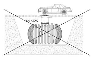
The tanks must not be installed in the ground water. If it is to be expected that the ground water could rise higher, even occasionally, as shown in the figure opposite, the ground water must be discharged via a drain line.
