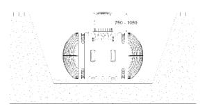
Max. covering heights with extension and drinking water telescopic dome shaft
