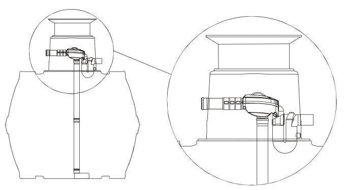
Optimax XL filter - internal (DN 150) For all tank applications with maxi domes for DN 150 connections
