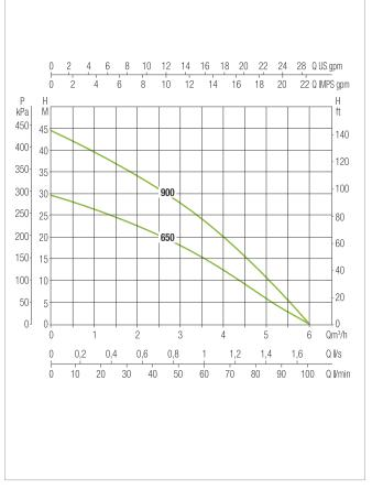
The performance curves are based on kinematic viscosity values =  $1 \text{ mm}^2/\text{s}$  and density equivalent to 1000 kg/m<sup>3</sup>. Curve tolerance according to ISO 9906.
