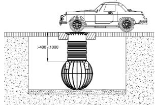
Cover heights with cast or HGV-bearing telescopic dome shaft
